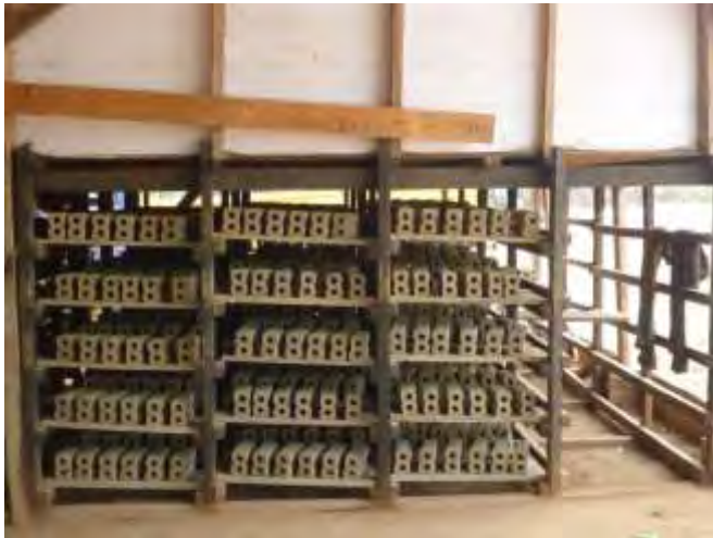
FIGURE 15 - DRYING GREEN BRICKS ON SHELVES
