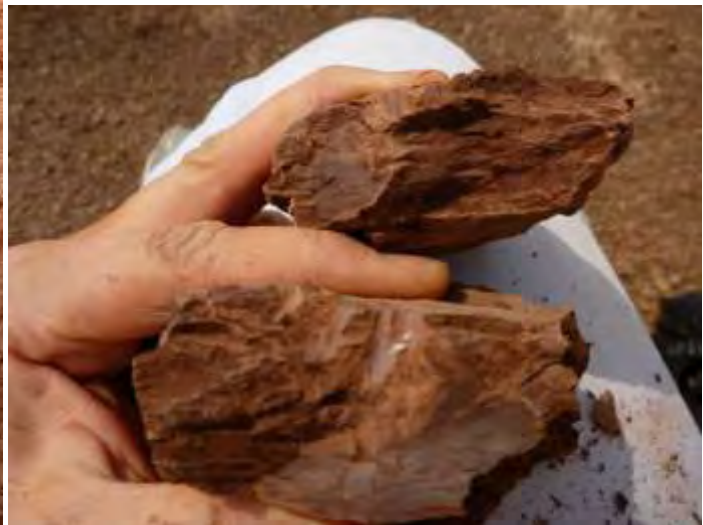
FIGURE 28 - COARSE GRAVEL-SIZED ROCK PIECES AT DEPTH
