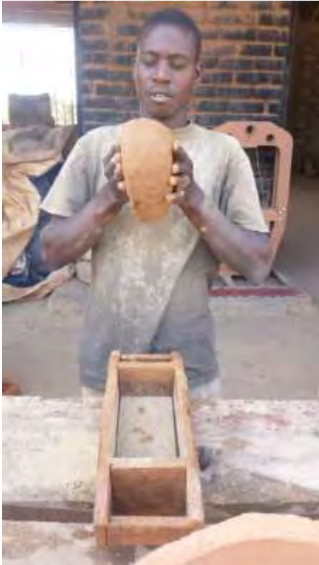
FIGURE 46 - HAND MOULDING BRICKS AT THE PHW FACTORY
