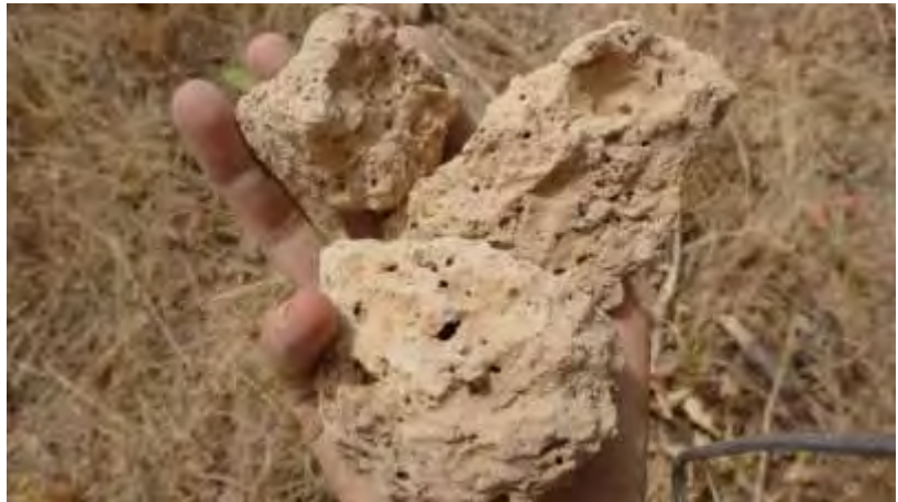
FIGURE 38 - POROUS TEXTURE OBSERVED IN LOAM AND TOP CLAY UNIT
