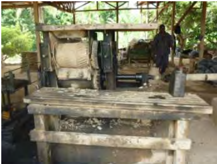
FIGURE 6 - PUG MILL USED TO MIX SOIL FOR BRICK MAKING
