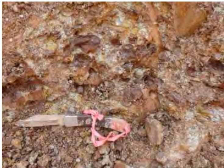
FIGURE 32 - IMAGE SHOWING DARK REDDISH BROWN ELLIPTICAL CONCRETIONS PRESENT AT DEPTH
