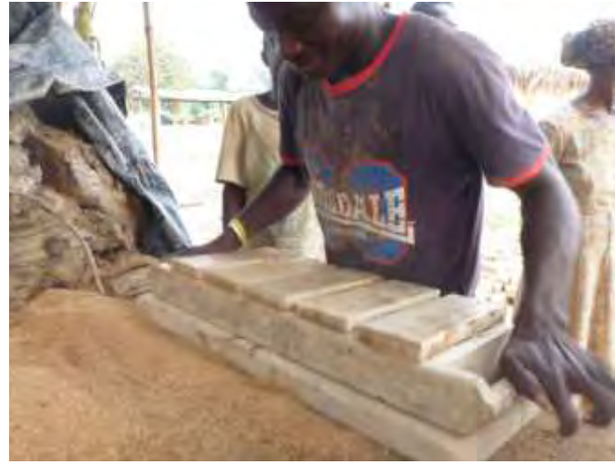
FIGURE 11 - HAND MOULDING GREEN BRICKS
