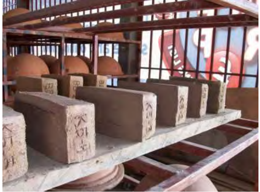
FIGURE 47 - DRYING GREEN BRICKS AT THE PHW FACTORY
