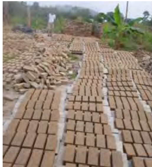
FIGURE 12 - GREEN BRICKS DRYING IN THE OPEN AIR
